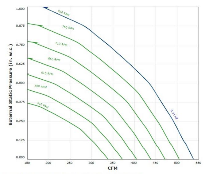
Max Sizeable RPM = 810 RPM. Curve shown extended beyond this point for reference only.
